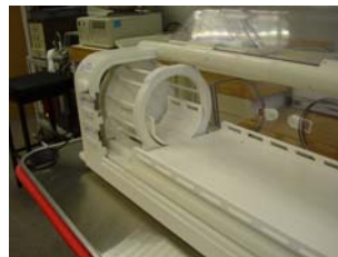
Fig 1. MR compatible incubator shown with the 'lid' open for access.
