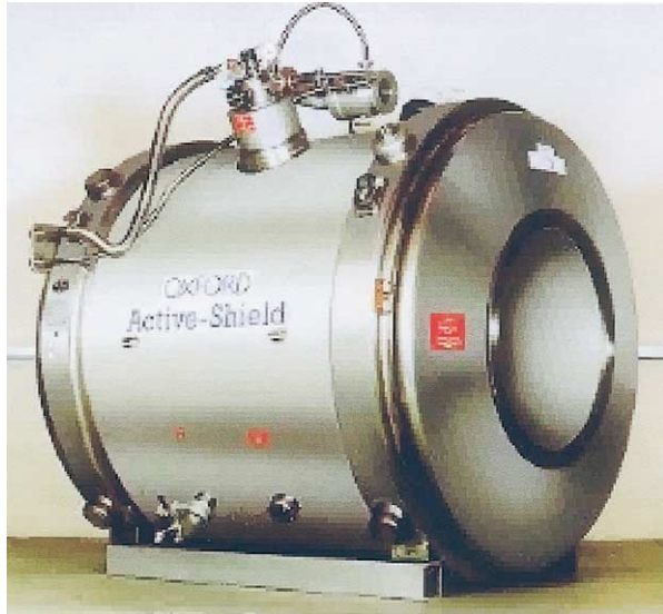
Figure 2. The superconducting magnet is an electromagnet in which current flowing in a circular direction in a coil of wire produces the intense, homogenous magnetic field required for high-quality imaging. Most MR magnets in hospitals are 1.5 Tesla or lower in strength; those used for research in infants can be up to 4 Tesla in strength. Image used with permission of Stephen Brick, MD, www.gcmradiology.com .
